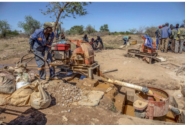
Worth its weight: An artisanal gold miner loads up a grinding, separating and sorting machine. (Photo: Bloomberg)
